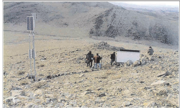
Seismic station in Mongolian mountains powered by solar energy.
